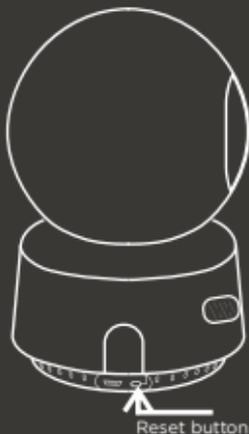
Press and hold the Reset button to restore your device to factory settings.
