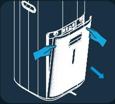
1. Remove the rear panel as shown here
